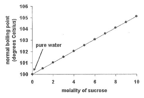
The graph above shows how the boiling point of a water/sugar mixture depends upon the concentration of sugar (sucrose) that is dissolved in the water. The concentration has units of "molality". If there is no sugar present in the mixture, then only water is present, and the molality is 0.
